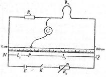
ference of 2.2 V. Calculate the work (a) You are provided with two resistance wires labelled: A and B, standard resistor  $R_x = 1 \Omega$ , metre bridge, cell of emf, E, key, Rheostat  $R_h$ , galvanometer and other apparatus.
